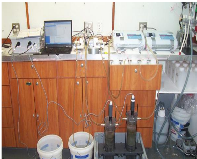
Figure 3-6. Dual-core Gust Erosion Microcosm System and Filtration System.
