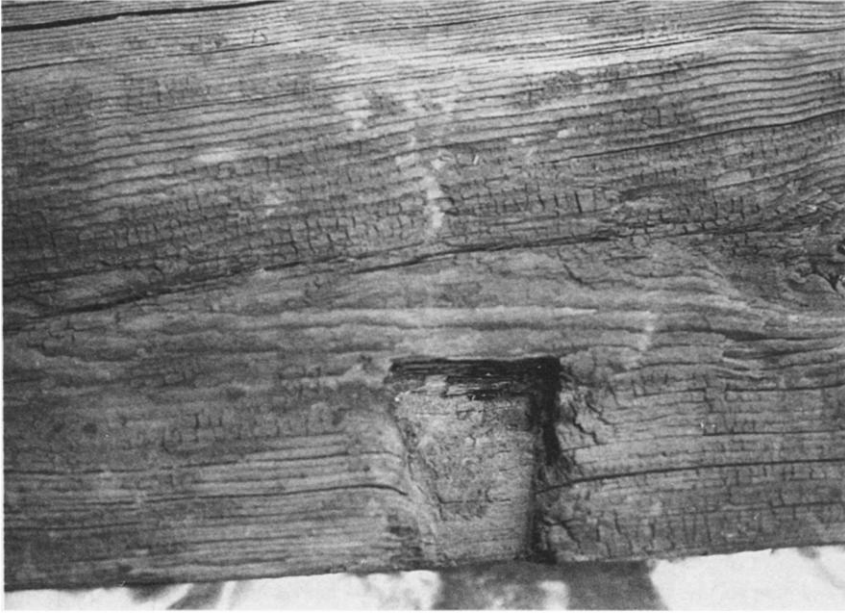
Fig. 2. Dovetail mortises in plank surfaces of the Dahshur boat in the Carnegie Museum of Natural History sometimes retain curious traces of former fastenings, and may have once been for lashings rather than wooden tenons. Unaltered mortises have smooth curves, as on the left side of this fastening; recut mortises have sharp, angled lines, as on the right side, but unusual depressions with rounded ends often remain visible in the bottom of the cut.
