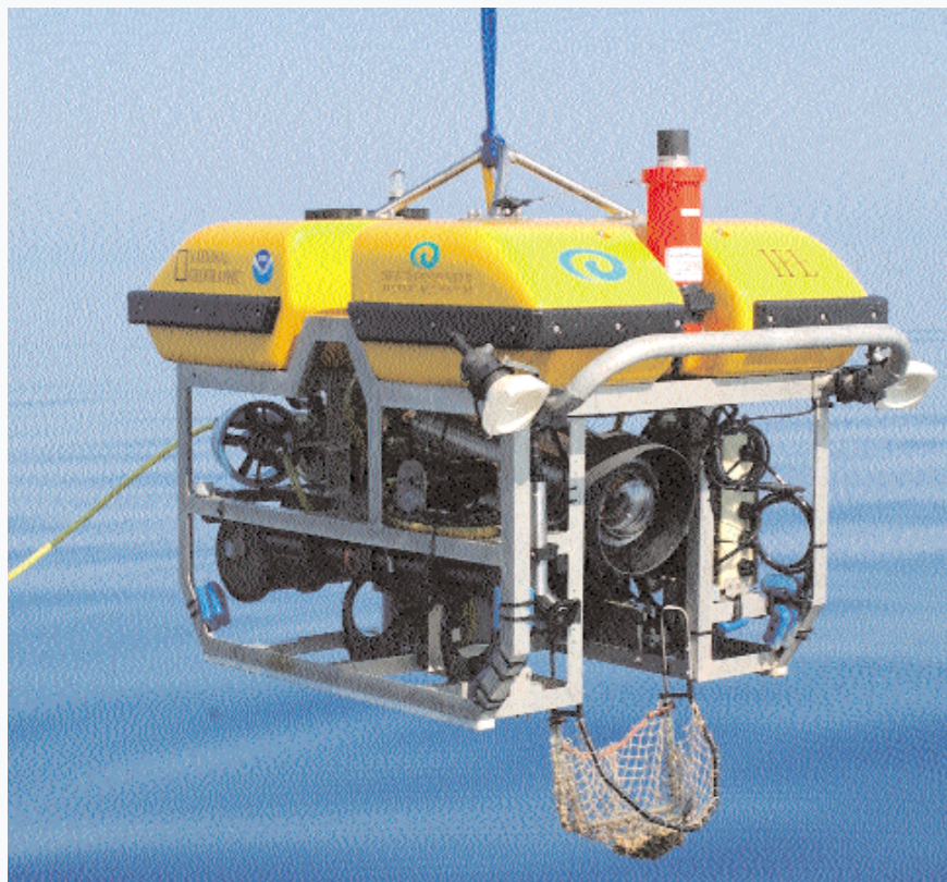
The ROV Little Hercules , with video and cameras, used to find and record shipwrecks in the Black Sea.
